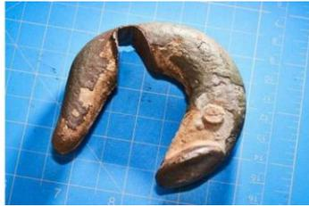
**A 3-inch C-hook could determine whether PG&E committed a crime.** On Nov. 8, 2018, a decades-old 3" C-hook broke, which led to a high-voltage electric line to fall, which sparked the Camp Fire that killed 85 people. Was the state's largest utility, which has hundreds of thousands of C-hooks, "negligent" in inspecting and replacing these hooks, and will some of its former executives face criminal charges for their role in wildfires? (Wholesale price of one C-hook: 56¢.)
